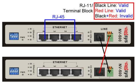
Figure 2.6.2 NV-500 line ports crossover connection
