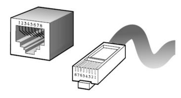
Figure A-1 Standard RJ-45 repectacle/connector
