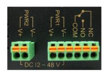
**STEP 1**: Insert the negative/positive DC wires into the V-/V+ terminals, respectively.
