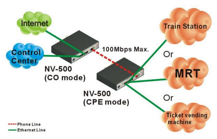
Figure 2.6 NV-500 point to point application
