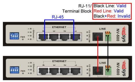
Figure 2.6.1 NV-500 line ports straight connection
